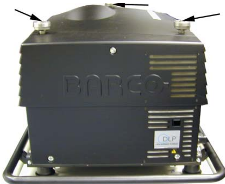
Image B-1 Removing stacking sockets
